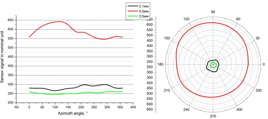
A fluoroplastic diffuser 2.5 mm thick was chosen. It completely suppresses the dependence of the photosensor, reduces the illumination of the photosensor, which will not allow you to get too large a signal in bright sun.
