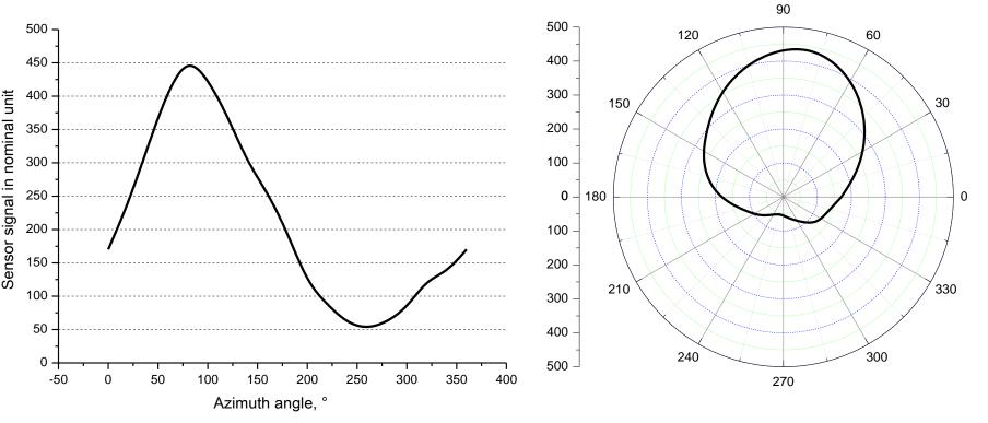
The azimuthal dependence is the dependence of the signal magnitude on the azimuthal angle of the radiation source with its constant zenith angle.
