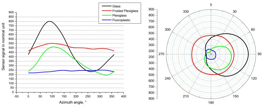
Based on the data obtained, it was decided to use fluoroplastic as a material for the diffuser.
